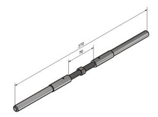
Assembly: Apply threadlocker high strength on the threads before tightening the wire
